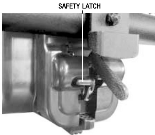
Figure 5. Freewheel Mode (Drive Disengaged)
